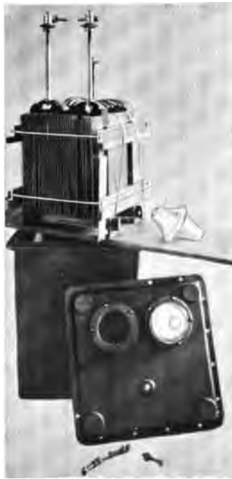
FIG. 30 a.—Large oil-condenser dismantled. [See p. 85.]
